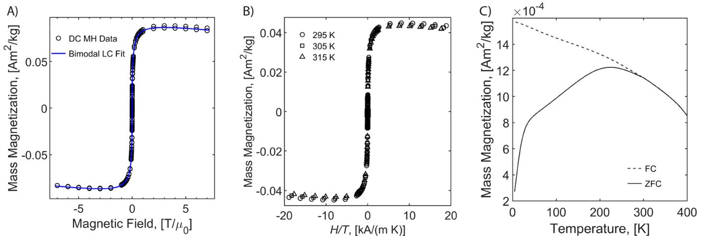
**Figure S5. Magnetic characterization of ferucarbotran.** A) MH curve at 300 K for ferucarbotran in water. B) MH curves at 295, 305, 315K for ferucarbotran in TEGMA C) ZFC/FC at 10 Oe for ferucarbotran in TEGMA.
