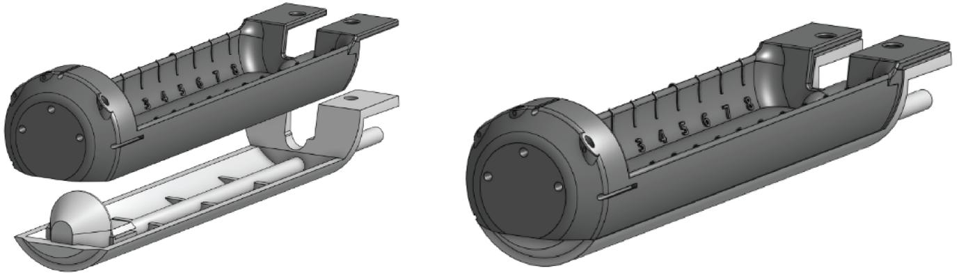
**Figure S4. Rendering of two-part animal bed assembly designed and 3D-printed for MPI animal studies.** The top and bottom animal bed parts (left) assemble a whole animal bed (right) that can be installed on Magnetic Insight's MPI scanner. The top part was designed with a flat bottom for ease of transfer of the mice from MPI to CT. The bottom part houses an integrated tubing system for isoflurane administration during imaging.
