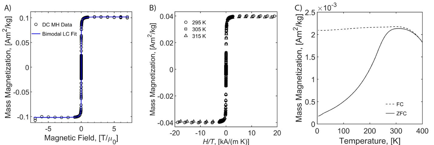
**Figure S6. Magnetic characterization of Synomag<sup>®</sup>-D.** A) MH curve at 300 K for Synomag<sup>®</sup>-D in water. B) MH curves at 295, 305, 315K for Synomag<sup>®</sup>-D in TEGMA C) ZFC/FC at 10 Oe for Synomag<sup>®</sup>-D in TEGMA.
