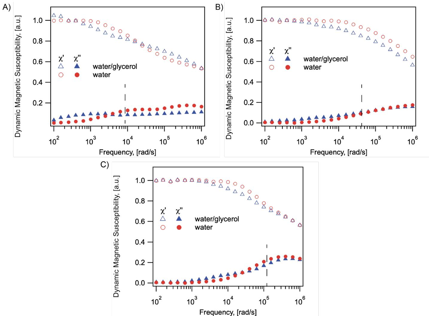
**Figure S8. Dynamic magnetic susceptibility characterization of relaxation mechanism for all three tracers. A) ferucarbotran. B) Synomag<sup>®</sup>-D. C) RL-1C. in water (red circle) or water and glycerol mixture (blue triangle, 65 wt% of glycerol). Dash line indicating peak frequency position for each particle assuming Brownian Relaxation dominant, based on their hydrodynamic diameter.**
