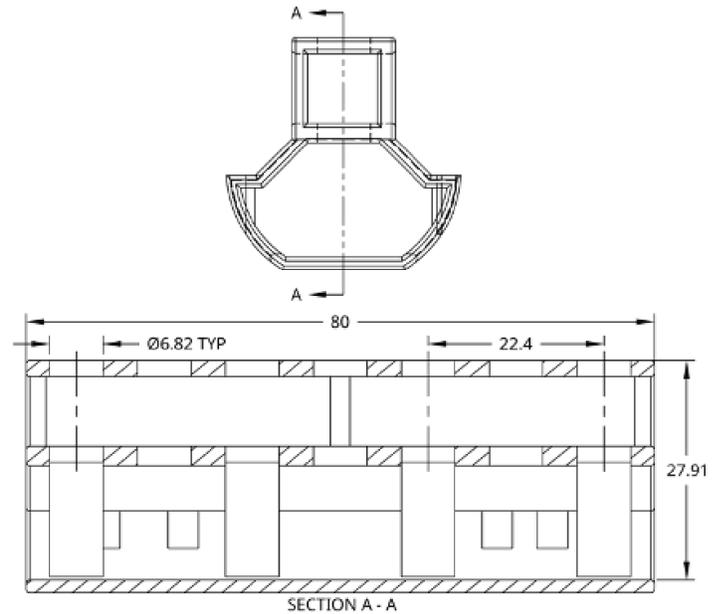
**Figure S3. Vertical 0.2 mL microcentrifuge tube holder designed and 3D-printed for MPI relax scan measurements.** The design accommodates 7 total tubes, with the entire lengths of 4 tubes able to be seen from a side view through exposed spaces. These 4 exposed spaces are 27.91 mm in vertical height with a center spacing of 22.4 mm.
