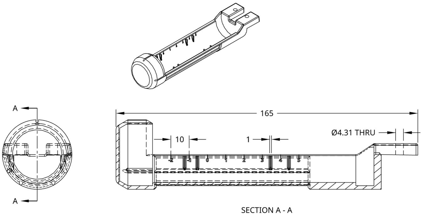
**Figure S1. Custom 3D-printed sample bed for phantom and SPION sample MPI studies.** Dimensions of this custom-designed sample bed were derived from Magnetic Insight's 45mL sample tube design and modified to fit the custom sample holders that were designed and 3D-printed for this study.
