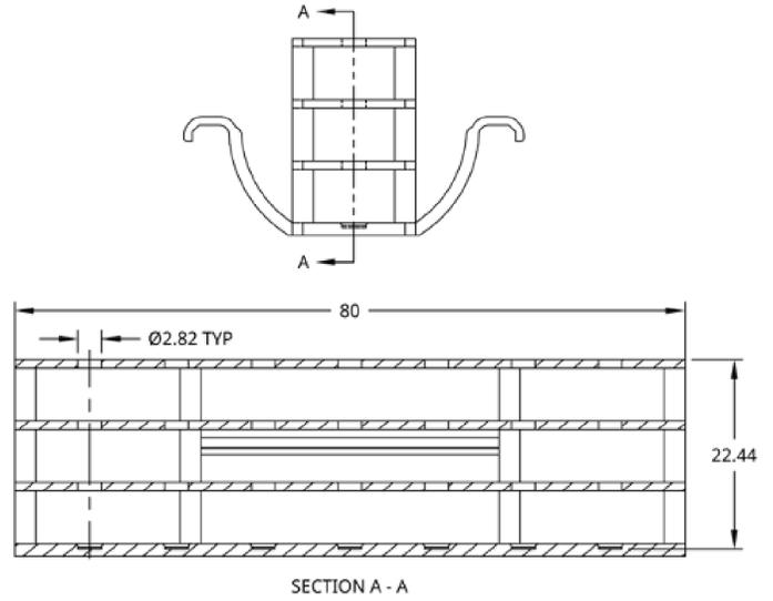
**Figure S2. Vertical capillary tube holder designed and 3D-printed for LoD studies.** Custom sample holders were designed in Onshape and 3D printed using Formlabs Clear V4 resin with the Form 3 SLA 3D printer.
