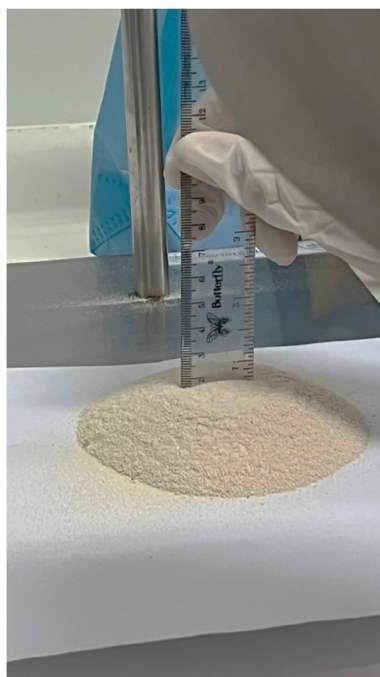
Figure 2. assessment of solid S-SNEDDS granules using the fixed-funnel method for angle of repose determination.
